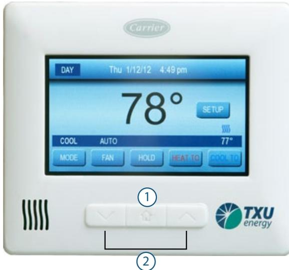
**Inactive Screen** – Provides a clean, uncluttered look. Screen will return to the Inactive mode after 60 seconds.
