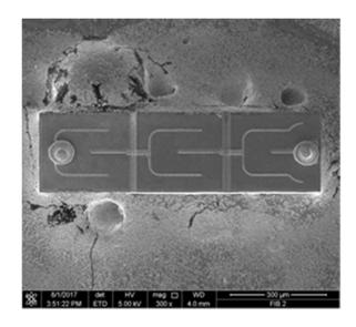
97. Below is a scanning electron microscope image of a pair of holes milled into the LED chip using a focused ion beam.
