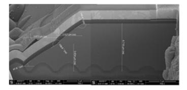
64. An insulation layer, which is comprised of SiO<sub>2</sub>, is arranged under a portion of the ITO current diffusion layer. This arrangement can be seen in the above images, where the SiO<sub>2</sub> is
