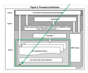
Hardware Abstraction Layer (HAL): this layer provides the low-level drivers and the hardware interfacing methods to interact with the upper layers (application, libraries and stacks). It provides a generic, multi instance and function-oriented APIs which allow to offload the user application implementation by providing ready-to-use processes. As an example, for the communication peripherals (I2S, UART...) it
